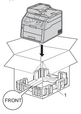
5 Place the packing material (2) marked "R" on the right of the machine. Place the packing material (3) marked "L" on the left of the machine. Place the AC power cord and printed materials in the original carton as shown in the illustration.
