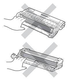
We recommend that you place the toner cartridge on a clean, flat, level, stable surface with disposable paper or cloth underneath it in case you accidentally spill or scatter toner. Turn the drum unit as shown in the illustration. Make sure the drum unit gear (1) is on the left side.
