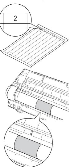
Turn the edge of the drum unit toward you by hand while looking at the surface of the suspected area.
