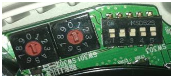
Figure 6.3 Close-up of Rotary Switches and Dip Switches
