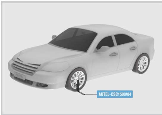
Figure 3-8 Auxiliary Tool Positioning
