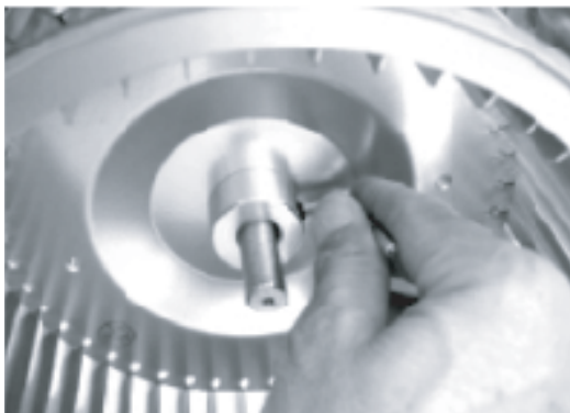
When replacing the fan motor, set it so that the model name label directs upward.
