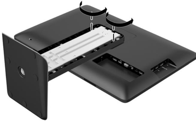
5. Lift the base up after 45 degrees to disengage the stand (1), and then pull the stand off of the monitor (2).
