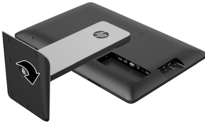
6. Tilt the stand base cover and first insert the edge away from the stand (1), and then press the cover down to snap the cover into place (2).
