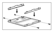
If you use a protection box (an additional accessory 1), the front airflow space of 2 mm and protective floor directly below the appliance are not necessary. You can not use the protection box if you install the appliance above an oven.
